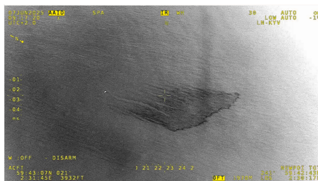
Fig. 6. Aerial IR (white-hot mode) photo of the MGO slick, 24 h after release. The thickest parts of the slick are found near the leading edge (towards the lower right). Photo taken from the surveillance aircraft LN-KYV.
