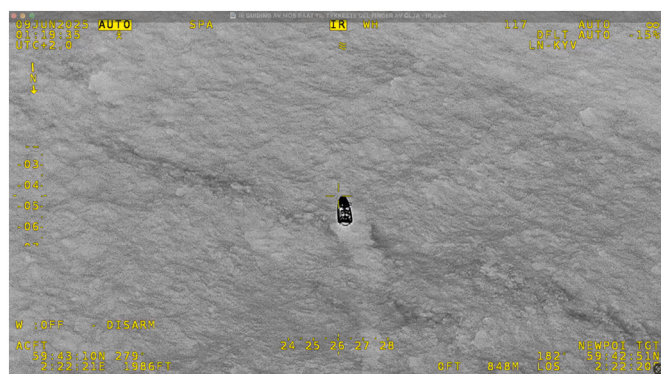
Fig. 11. IR photo (white-hot mode) taken from LN-KYV, showing the Oseberg slick and workboat doing surface sampling, 16 h after release. No continuous thick oil was visible at this time.
