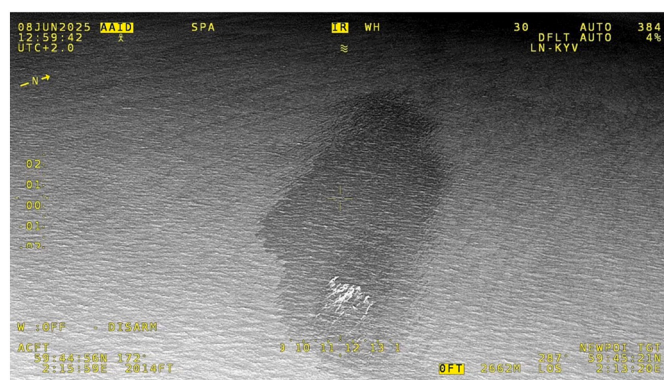
Fig. 10. IR photo (white-hot mode) of the Oseberg slick 4 h after release, taken from LN-KYV. The white area indicates thicker parts of the slick.
